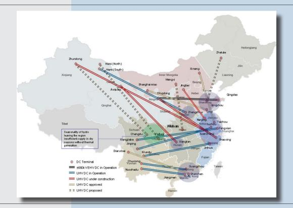
Figure 3: UHV DC transmission lines
